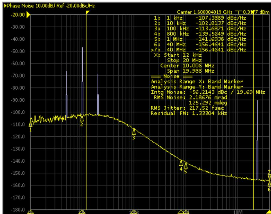
The location of the first-order integer boundary spurs is determined by the difference between the VCO frequency and the nearest harmonic of the reference frequency (or PFD frequency). In the second case example above, that difference is  $3200.01 - (100 * 32) = 10$  kHz.
