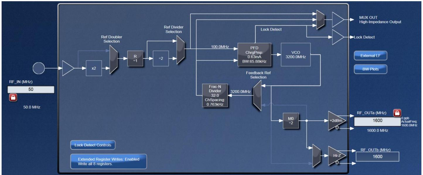
**Figure 3. 8V97053 Feedback Divider Settings for 1.6 GHz Output using a 100 MHz PFD Frequency**
