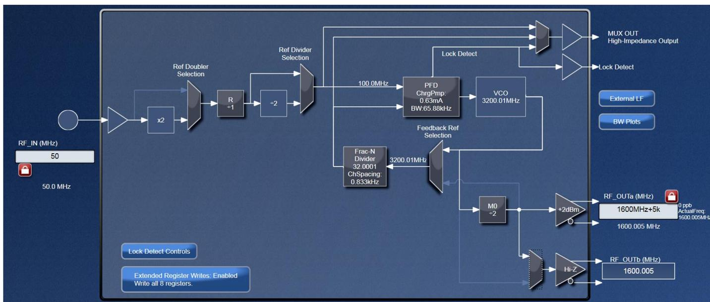
**Figure 6. 8V97053 Feedback Divider Settings for 1.6 GHz + 5 kHz Output with 100 MHz PFD Frequency**
