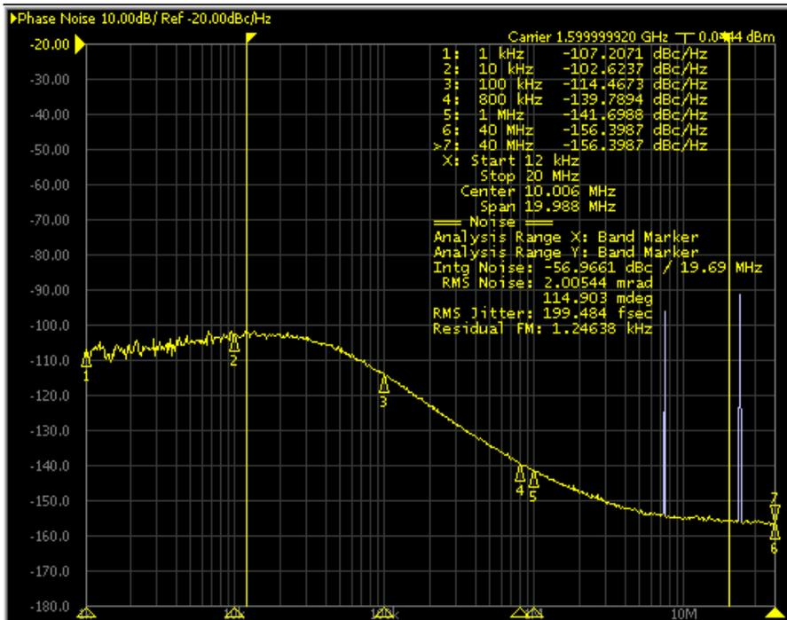
In the second case, an output frequency of 1.6 GHz + 5 kHz is desired, so the PLL is forced into a fractional mode. See Figure 5 for the configuration and Figure 6 for the feedback divider settings. The fractional value of the divider is now non-zero and is very small because the additional output frequency step is very small. In this example, using a calculation similar to the first case, the desired feedback divider value is 32.0001, which is very close to the integer value 32.
