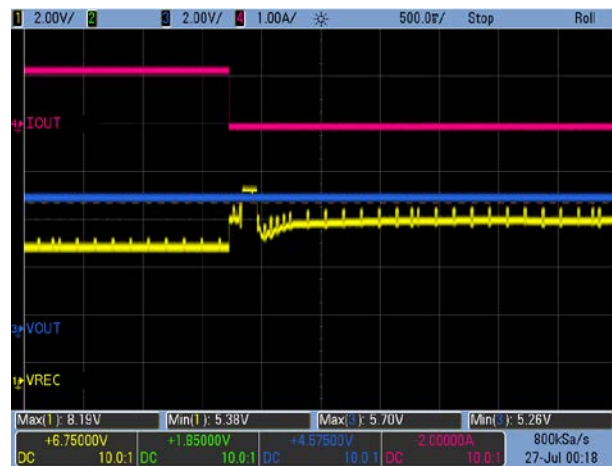
Figure 12. Load Transient: V OUT = 5V, 1.2A → 0A
