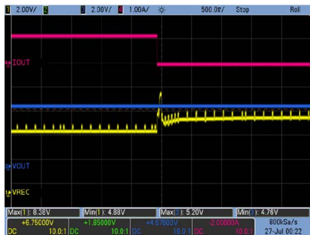
Figure 12. Load Transient: V OUT = 5V, 1.2A → 0A
