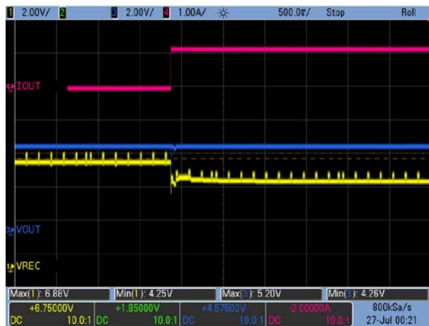
Figure 11. Load Transient: V OUT = 5V, 0A → 1.2A
