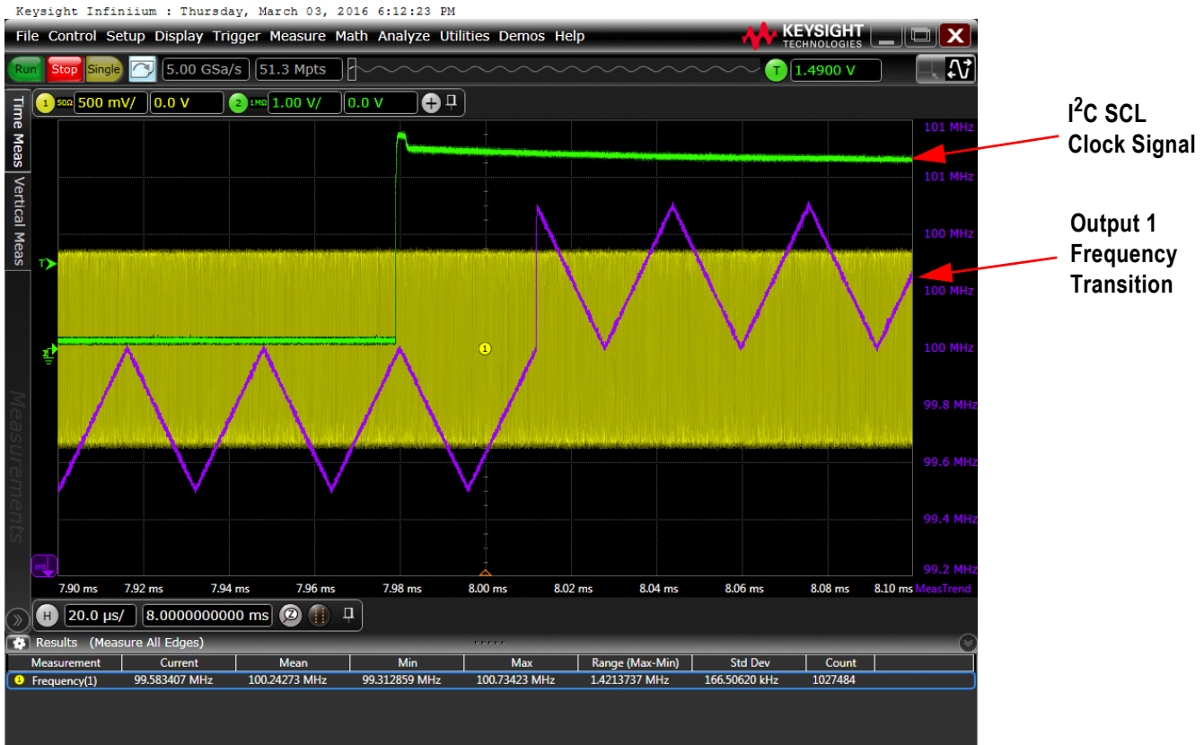
Figure 6. Oscilloscope Image of Output Frequency Transition
