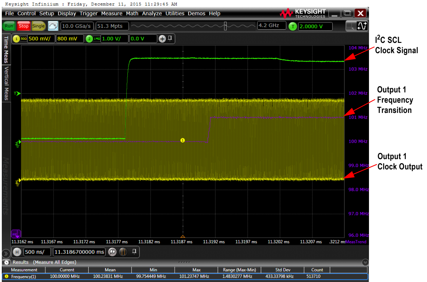
Figure 4. Frequency Transition from 100MHz to 101MHz
